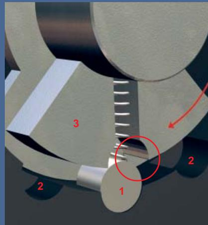
As a break-in is attempted, the security bolts (1) are forced into special notches (2) in the housing by a second coupling element (3).
